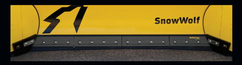
No more "just scraping by." Like other traditional sectional plows, the ActivEdge has multiple sections that move, or float, over obstacles or uneven surfaces. Since they conform more closely to the surfaces, regardless of contours or obstacles, the result is a cleaner scrape than is possible with a one-piece plow.
